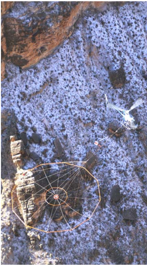
Geotech Ltd. flies a VTEM survey for Quaterra on the Arizona Strip uranium project. Courtesy: Quaterra Resources
